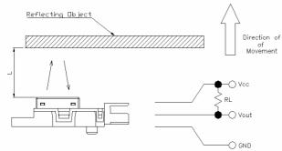
\*6 : Maximum detection distance measuring method.
